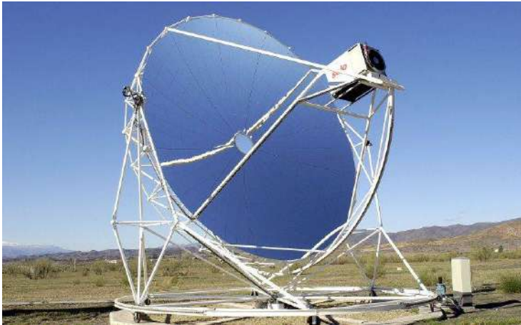
Gambar 6.12 Model solar dish kapasitas 10 kW (EuroDish) [63]
