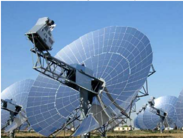
Gambar 6.11 Model baru Stirling Energy Systems kapasitas 25 kW [62]
